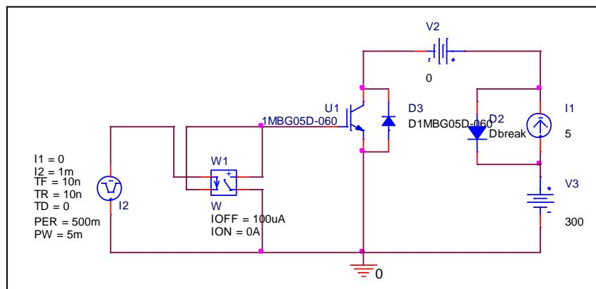
Test condition:  $V_{CC}=300$  (V),  $I_C=5$  (A),  $V_{GE}=15$  (V)
