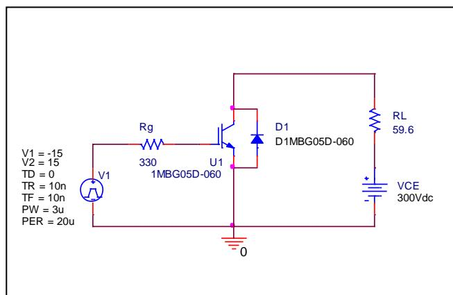
Test condition:  $I_C=5$  (A),  $V_{CC}=300$  (V)
