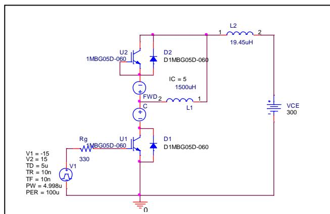
**Test condition: Vcc=300 (V), Ic=5 (A), di/dt=-15A/usec**
